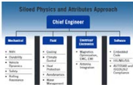
*In the automotive industry, mechanical strength of a brake rotor is studied separately from air flow that cools the brake, for example. Single-physics simulation studies a sole physical effect in isolation. This approach does not recognize potential failure modes when phenomena intersect. Furthermore, simulation in various disciplines is performed sequentially instead of in parallel, lengthening the development cycle.*
