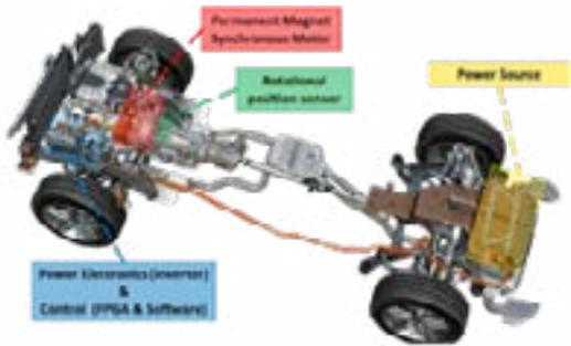
Systems modeling and simulation is applicable to a new age of products in the automotive industry. The system-level models for this electric powertrain system include ANSYS Simplorer (a platform for assembling and testing performance of virtual system prototypes), ANSYS Maxwell (2-D and 3-D electromagnetic simulation), ANSYS Q3D Extractor (parasitic extraction tool) and ANSYS SCADE (for creating and optimizing embedded software).
