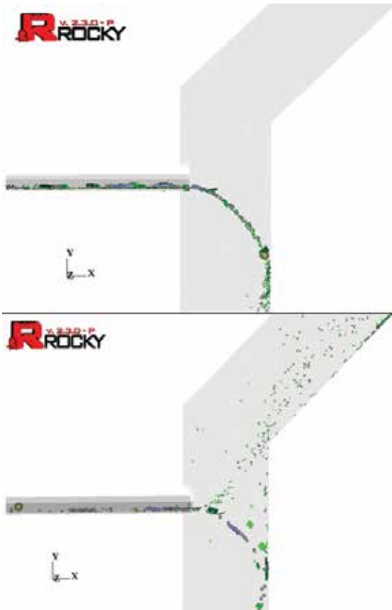
Figure 2. Comparison between pure DEM (above) and one-way CFD-DEM approaches (below) for a windshifter case
